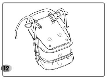
• Fit the ends of the seat back wire into the **outside** holes in the seat tubes.
